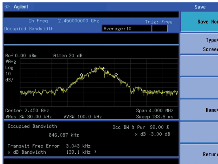
Figure 3. OBW available as a convenient one-button measurement on the N9320B
